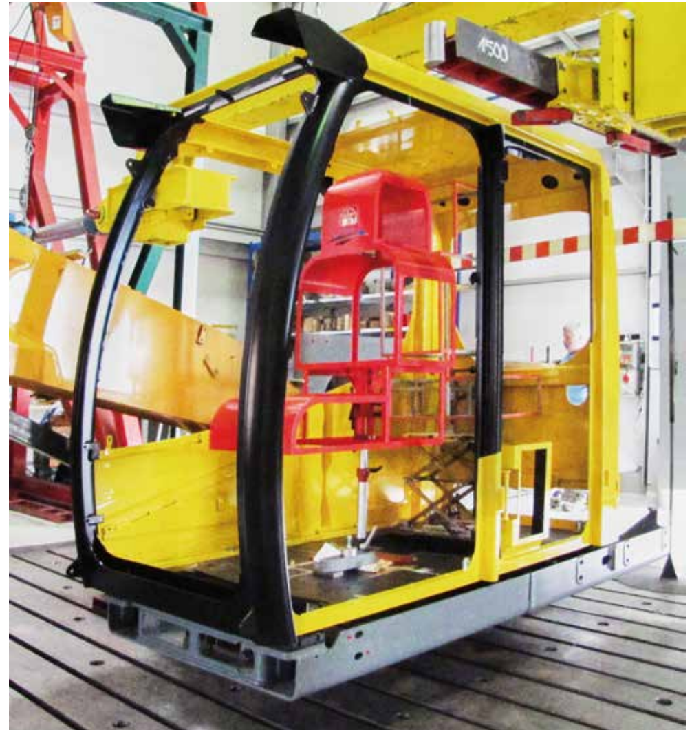
ISO tests for ROPS/FOPS safety structures
