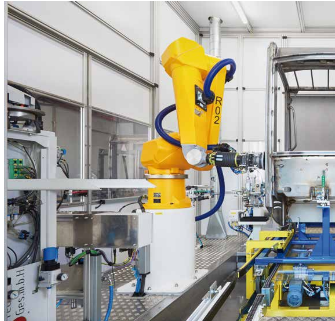
Full-automated grinding robot for cabin structures
